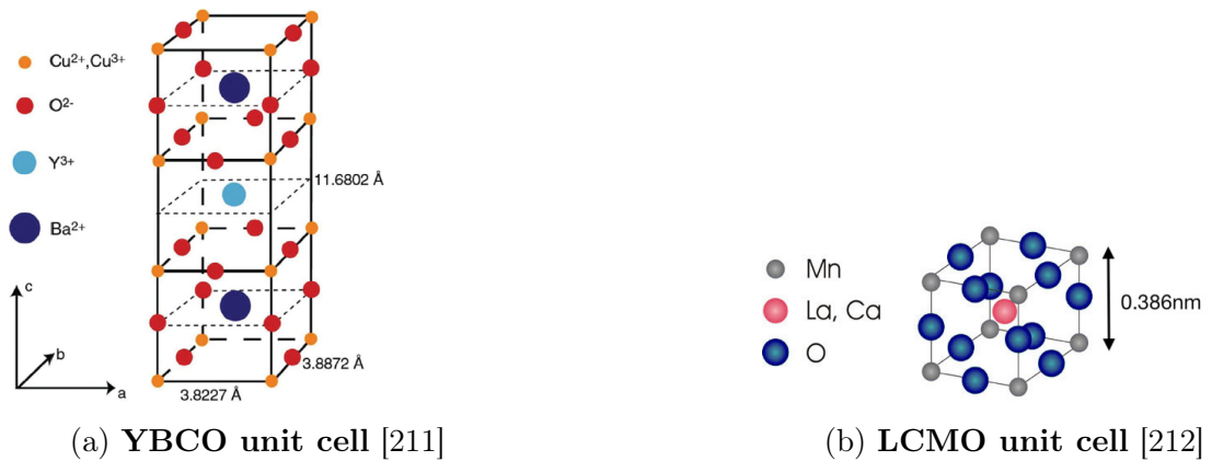
Figure 3.2: Unit cells of YBCO and LCMO
